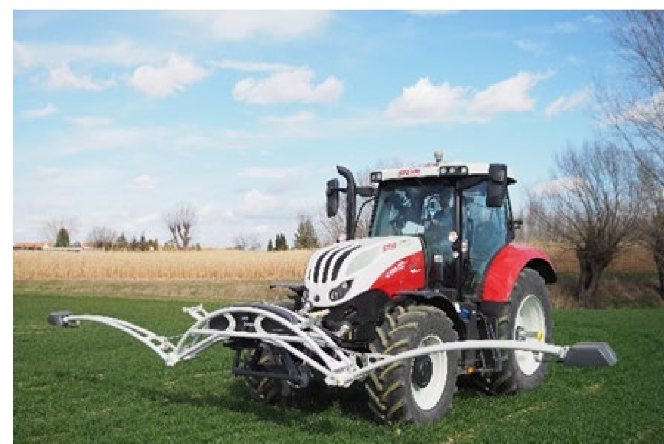
Picture 2. Crop sensor used for VRNA
