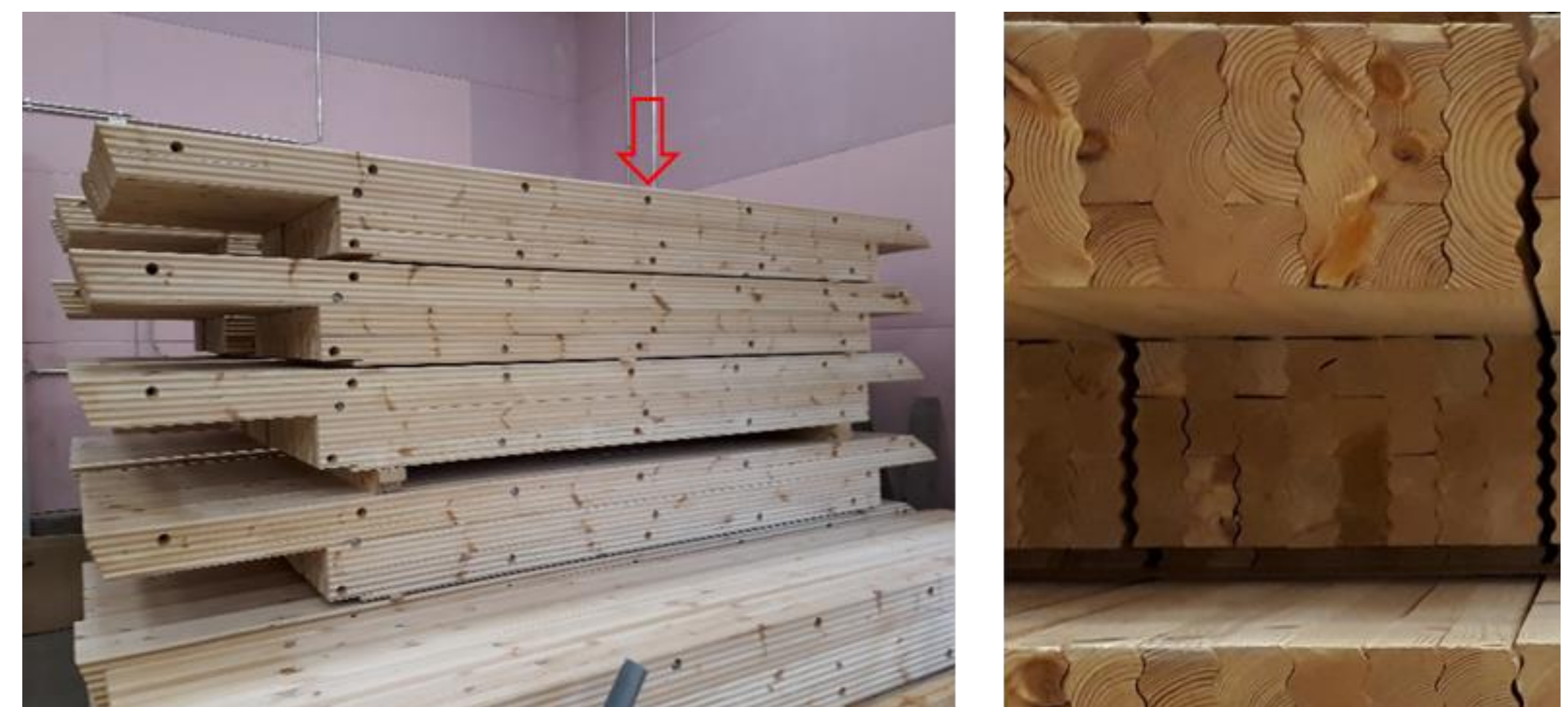
Figure 1. One of the assessed case products. Stack of pre-assembled WLT elements (left) and a detail from an element's end (right). Red arrow points to a duct for threaded rods that tie the boards and elements as a WLT wall structure. Pictures: Tarmo Rätty
