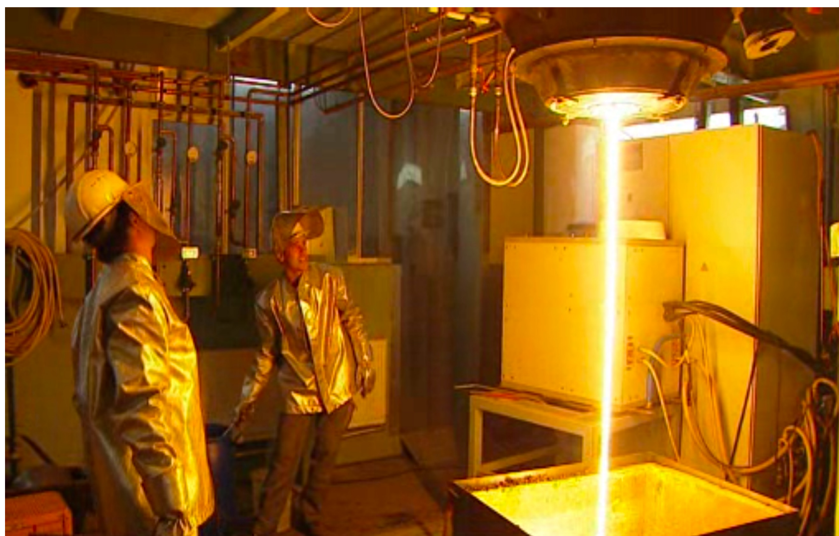
Tapping of Flash Reactor. Picture: Alfred Edlinger / Metallic and Inorganic Technology
