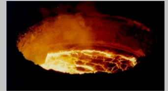
Molten steel in the ladle
